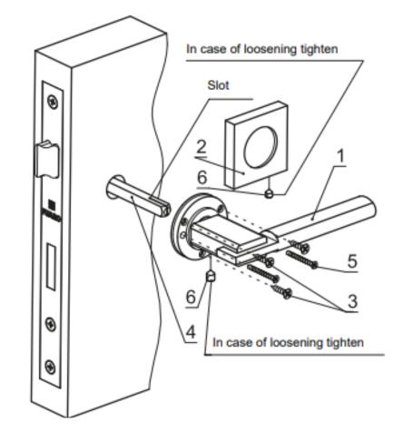
Place the connecting square (4) in the swivel socket of the lock. Make sure the square slot is positioned correctly.
